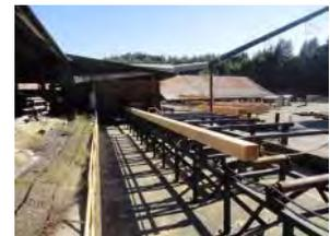
▲ **New Sail Cross Arms**—A long lead time is required on the purchase of the new set of timber sails so they were ordered in May. Main stock lengths are 67' in length and 12x12 In section. The timbers were transported from Oregon to Kentucky in August where they are being dried at Hasset's shop to an "air dried" moisture content, then treated with preservatives.
